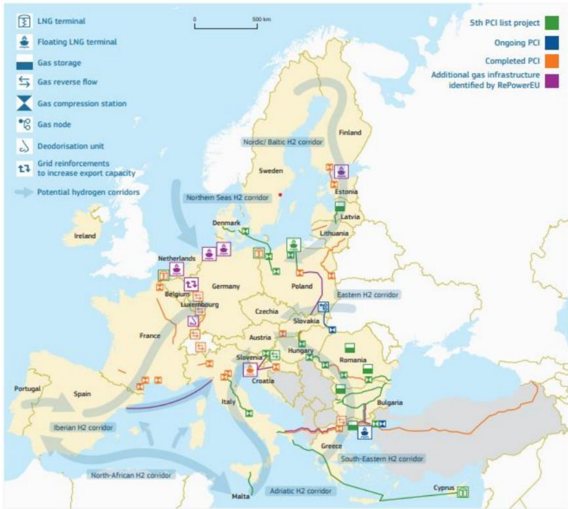
Figure 21 Indication of potential hydrogen corridors across EU, according to REPowerEU Plan
